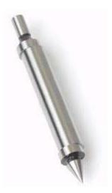
Edge finders locate the edge of the workpiece. Center finders locate the center of existing holes. Wigglers locate the intersection of scribed lines on the workpiece.
