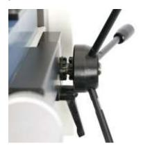
Fine feed disengaged
