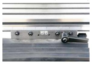
X-axis gib adjusting screws
