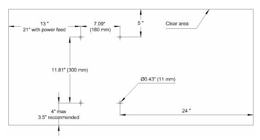
Mount the mill to the workbench with 3/8" or 10 mm bolts. The bolts should be about 1" (25 mm) longer than the thickness of the workbench. Use fender washers on the underside of wooden benches to prevent the nuts from pulling through.
