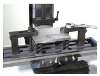
When clamping with step blocks and clamp bars, the end of the clamp bar on the step block should be just a little higher than the end on the workpiece. This ensures that the end of the clamp bar makes contact with the workpiece. The stud should be located as close to the workpiece as possible so that the majority of the clamping force is exerted on the workpiece and not the step block.
